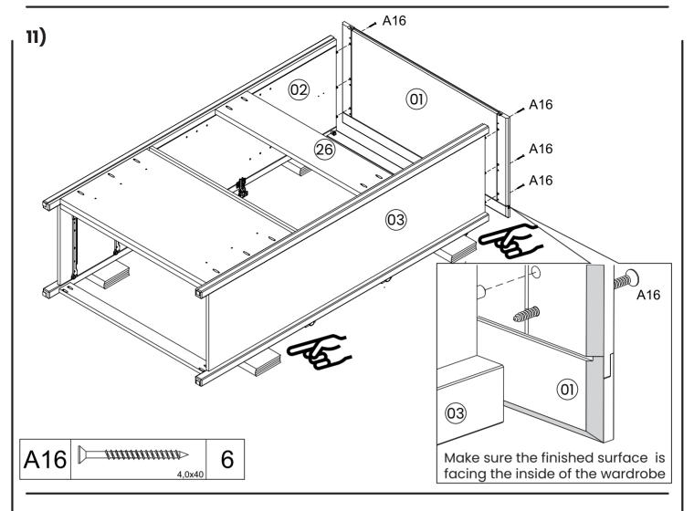
Make sure back panels are perfectly aligned with side panels and top and there are no gaps.
