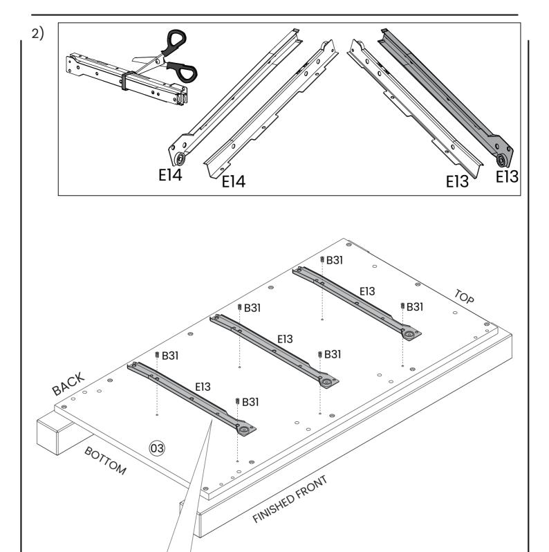
Glide wheels should be positioned towards the front and bottom of the side panel.
