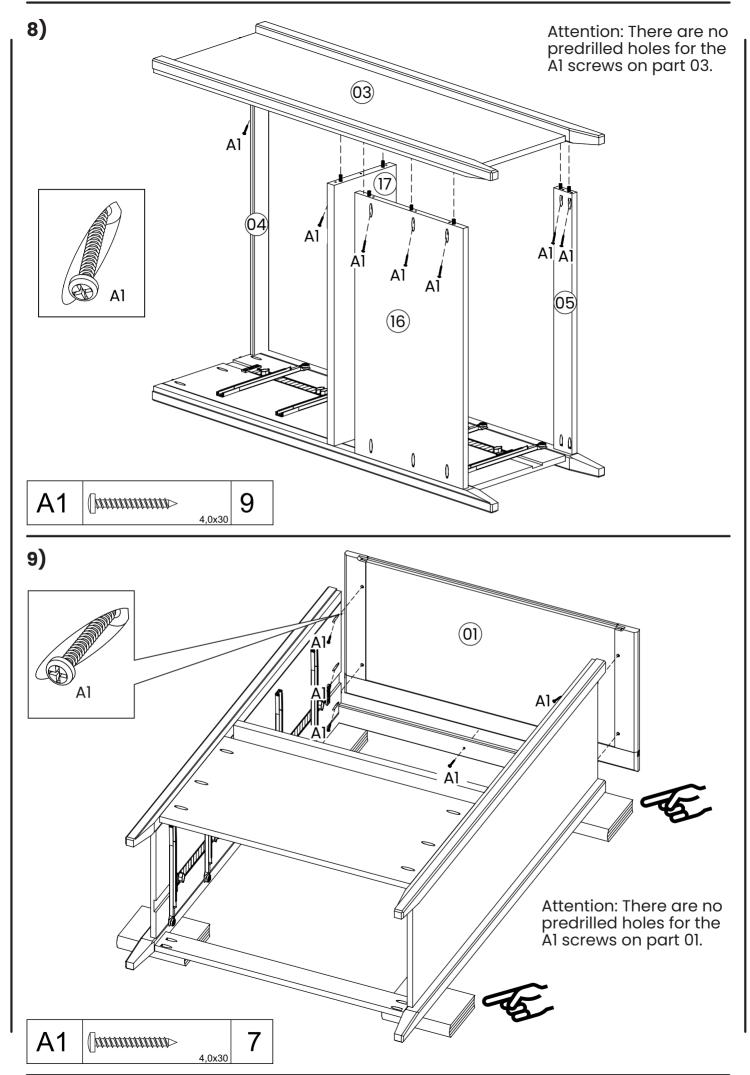
Make sure back panels are perfectly aligned with side panels and top and there are no gaps. 10) Gap present G1 رِّ G1 07 G1 No gap ์G1 🖁 G1 4 10x10 11) Gap present G1 G1 G1 07) No gap G1 4
