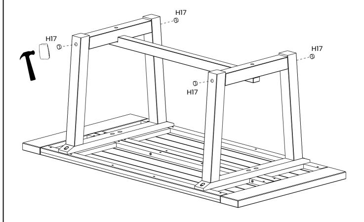
Tip: Use a rubber mallet or a piece of wood to protect the finish when hammering the wood cap
