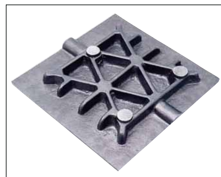
Diagonal cross-ribbed webbing on the underside for maximum rigidity & minimum deflection
