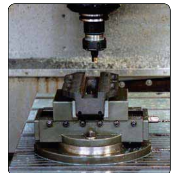
Self Centering Vice being used to mill key ways in the center of the casting
