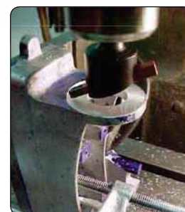
Fly Cutter Holder with tool being used for face machining of a job on a vertical milling center
