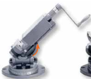
Movement along the first angular slide, 0-90°
