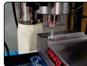
Edge Finders being used to locate the edge of a job held in a milling vice
