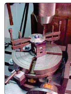
Parallel Clamps being used to hold a job for precisiondrilling operation
