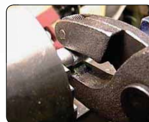
Knurling Tool Holder-being used for doing knurling on a job fitted onto a lathe machine
