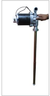
Now connect the Suction Tube to the pump inlet. Hand tighten Lift the Pump with Hand.
