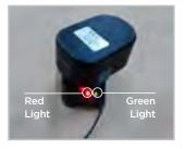
When battery is fully charged, only green light remain steady and red light turns off.
