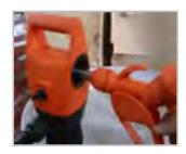
Push a fully charged battery into the Battery holder.
