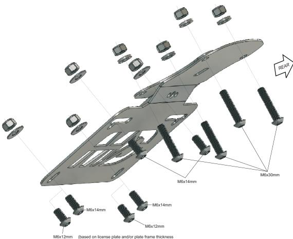
determine the clearance and use the appropriate bolt)
