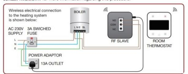
Upon completion of wiring for either wired or wireless versions refit the front cover housing and secure with the supplied hex screw. Refer to User guide for programming and operation.
