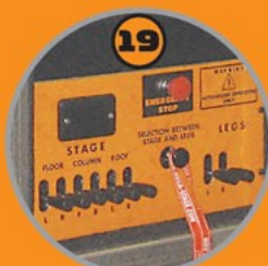
Main hydraulic controls with Emergency kill switch
