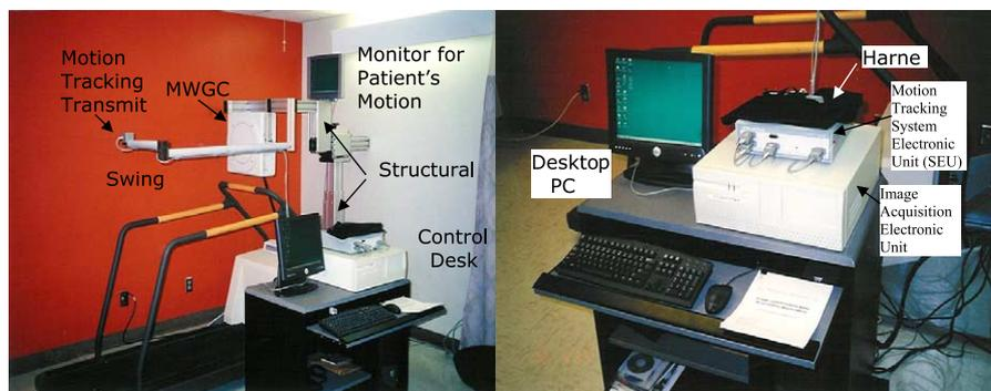
**Figure 1.** Setup of MWGC, motion-tracking device, and treadmill at the University of Alabama at Birmingham. The *left panel* shows the treadmill unit with the head of the MWGC attached to it. The motion-tracking transmitter is attached to a swinging arm. The monitor on top displays the position of the heart. The *right panel* shows two electronic units, one for motion tracking and the other for image acquisition.
