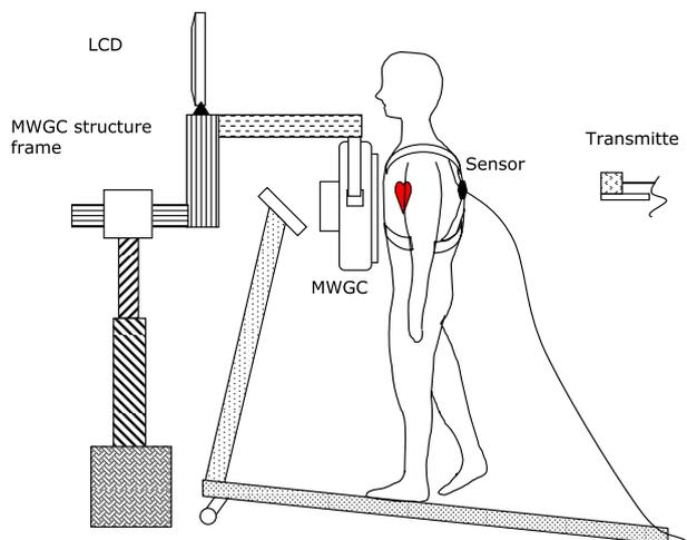
**Figure 2.** Schematic illustration of motion-tracking devices during exercise. By use of the transmitter and sensor, real-time position information is obtained.
