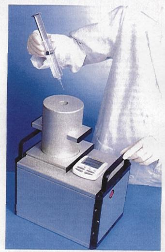
FIGURE 3. Clinical 62Zn/62Cu generator with collection syringe ready for insertion.
