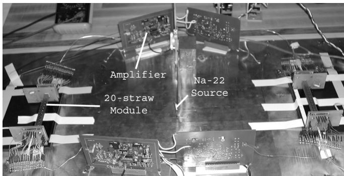
Fig. 4. Experimental setup used for coincidence detection of Na-22 line source. The paralleling of the 20 anode signals through termination resistors into a single amplifier is readily seen. The entire readout was done using 4 amplifiers seen at the center, whose outputs were digitized using an oscilloscope (Lecroy LT344, 500 MS/s).
