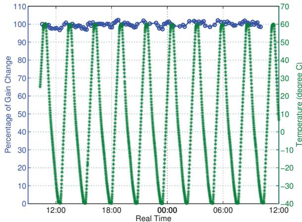
Fig. 8. Temperature cycling of straw detectors.
