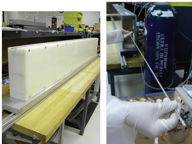
Fig. 4. Polyethylene moderator block (left), and 200 cm long straw detector (right) being inserted into one of the 171 holes machined into the polyethylene.
