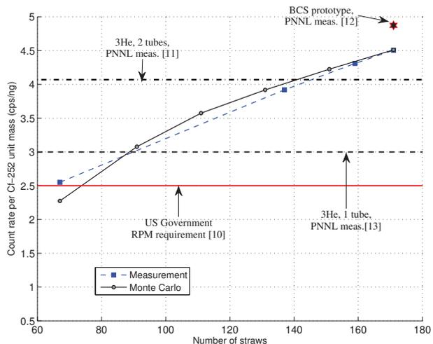
Fig. 6. Measured and predicted (Monte Carlo) count rates in the prototype monitor, as a function of the number of straw detectors, for a moderated  $^{252}\text{Cf}$  source at 2 m; PNNL measurements of the BCS prototype and of  $^3\text{He}$ -based RPMs are indicated.
