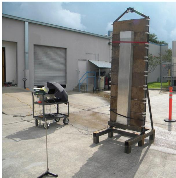
Fig. 5. The prototype detector during testing outdoors. The detector is supported in front of a 1-inch thick steel plate, with its center 1.5 m above ground. A  $^{252}\text{Cf}$  source is supported on a tripod 2 m in front of the detector face.
