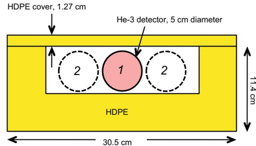
Fig. 1. Typical design and dimensions of a neutron detector for radiation portal monitors, with a single  $^3\text{He}$  tube (dashed circles show possible tube locations in the two-tube design). The high-density polyethylene box has a height of 215 cm. The tube is pressurized to 3 atm.
