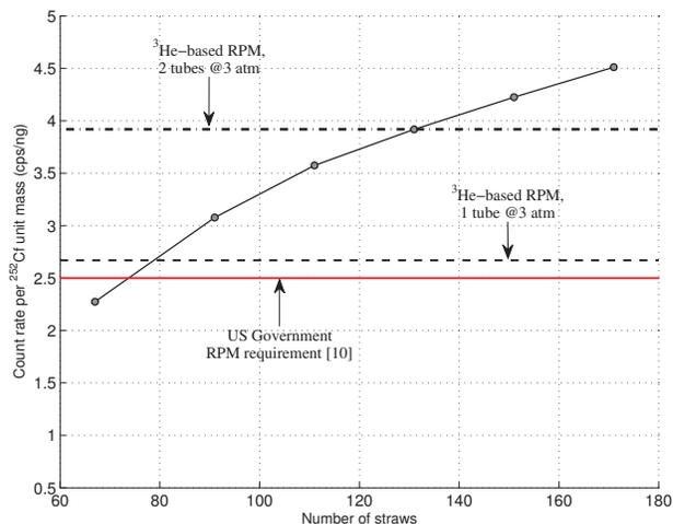
Fig. 3. Predicted count rate in BCS-based detector design of Fig. 2, as a function of the number of straws, for a moderated  ${}^{252}\text{Cf}$  source at 2 m; and predicted rates for the  ${}^3\text{He}$ -based design of Fig. 1, with 1 and 2 tubes.
