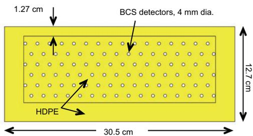
Fig. 2. RPM neutron module design based on BCS detectors. Straws are distributed within the central area of high-density polyethylene. The outer dimensions are those typically encountered in  ${}^3\text{He}$ -based designs (see Fig. 1). Each straw detector is 2 m long.
