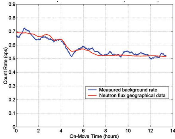
Fig. 9. Background count rate measured in the long-range detector during a road trip from Oak Ridge, TN to Houston, TX. The red line is an estimate of the cosmic neutron flux at each corresponding geographical location, based on equations published in [14].
