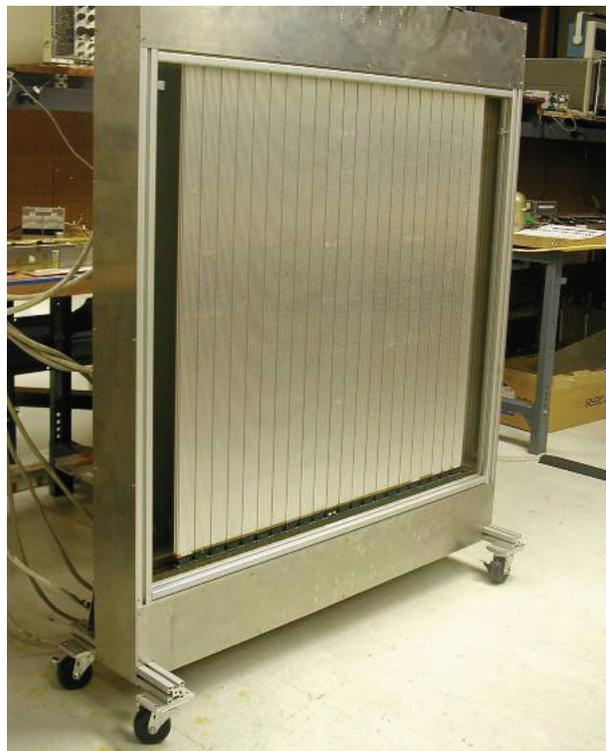
Fig. 7. Prototype neutron imaging  $1 \text{ m}^2$  detector (left), and testing at the HFIR neutron science facility (Oak Ridge, TN).
