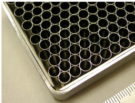
Fig. 3. One centimeter long straws, each lined with a thin layer of  $^{10}\text{B}_4\text{C}$ , are close-packed to form a neutron collimator.
