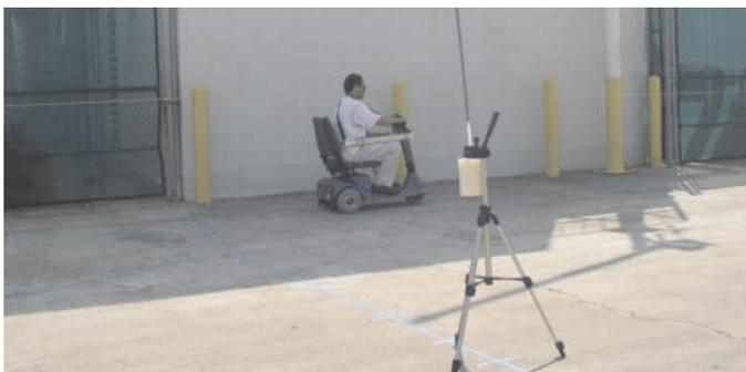
Fig. 4. Testing with the monitor carried by the cart operator, traveling at various speeds. The neutron source is visible in the foreground, mounted on a tripod and inside a thermalizing polyethylene cylinder.
