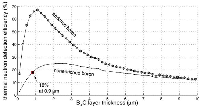
Fig. 8. Predicted thermal neutron detection efficiency, for a natural and <sup>10</sup>B-enriched boron carbide layer of increasing thickness. The two curves reach their maxima at different layer thicknesses. The efficiency measured in the prototype monitor is indicated by the square symbol.
