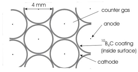
Fig. 1. A close-packed array of copper-walled straws, lined with  $^{10}\text{B}_4\text{C}$ , is proposed for the detection of thermal neutrons.
