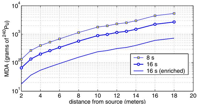
Fig. 10. Estimate of the minimum amount of <sup>240</sup>Pu detectable in the proposed monitor, for the integration times indicated. Results were based on measurements using a moderated <sup>252</sup>Cf source. The lower curve corresponds to a prediction for enriched boron carbide. The false alarm rate was less than 0.5 alarms/hour, and the sensitivity was 90%. MDA: minimum detectable amount.
