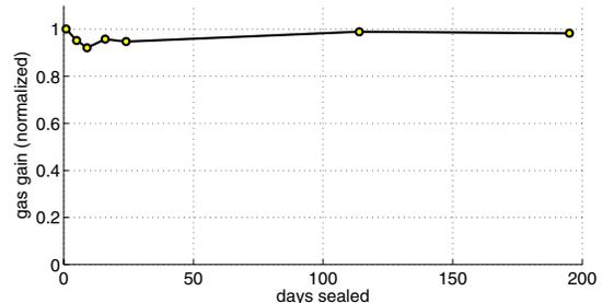
Fig. 7. Gas amplification was tracked in the prototype monitor using the 8 keV full energy peak of the  $^{241}\text{Am}$  energy spectrum (see Fig. 5). On day 1, the amplification factor was 2200.
