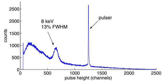
Fig. 5. Pulse height spectra collected in the prototype monitor, operated at 1000 V, and irradiated with a  $^{241}\text{Am}$  source.
