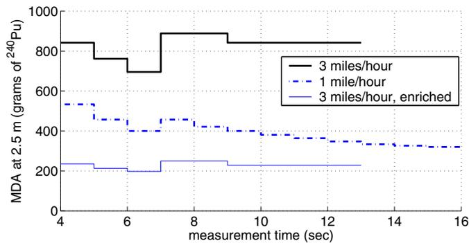
Fig. 11. Estimate of the minimum amount of  $^{240}\text{Pu}$  at 2.5 m, detectable in the proposed monitor, traveling at the speed indicated. Results were based on measurements using a  $^{252}\text{Cf}$  source. The lower curve corresponds to a prediction for enriched boron carbide. The false alarm rate was less than 0.5 alarms/hour, and the sensitivity was 90%. MDA: minimum detectable amount.
