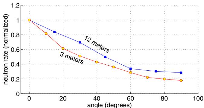
Fig. 9. Angular response measurements.
