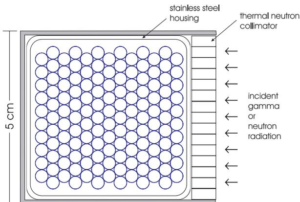
Fig. 2. Cross-sectional diagram of prototype monitor, showing the straw detector array, stainless steel housing, thermal neutron shield and collimator.
