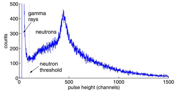
Fig. 6. Pulse height spectra collected in the prototype monitor, operated at 1000 V, and irradiated with a  $^{252}\text{Cf}$  neutron source.
