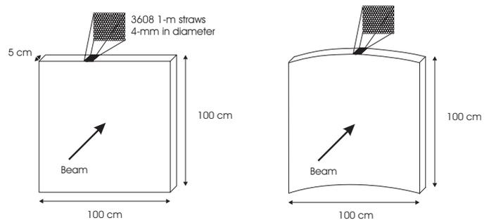
Fig. 1. Neutron area detectors composed of dense-packed  $^{10}\text{B}_4\text{C}$  lined straws, showing a flat panel configuration (left) and a curved panel (right) whose curvature matches the radius of the scattering geometry.
