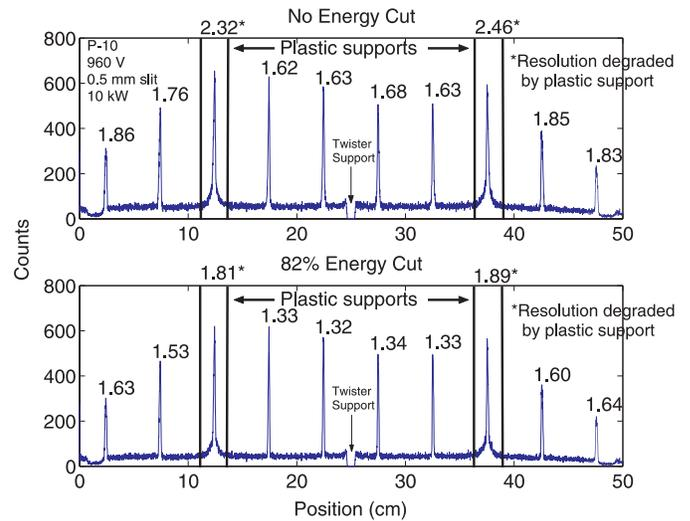
Fig. 10. (top) Position spectra collected in a single, 50 cm long straw, 2 mm in diameter, using a slit collimator. (bottom) The same spectrum with an upper discriminator level that rejects high energy events (18% of events rejected), resulting in improved resolution. Note the peak broadening in the two peaks positioned over plastic supports, and the clean, narrow inefficient spot in the center, produced by the central wire support.
