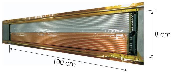
Fig. 3. Aluminum (top) and copper (bottom) prototype detector modules, close-packed to form a  $100 \times 8 \text{ cm}^2$  panel. Neutrons are incident on the face shown. The depth dimension, in the direction of irradiation, is 1.73 cm.
