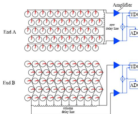
Fig. 4. Electronics setup for straw readout, showing circuitry connected to the two respective ends of each module.
