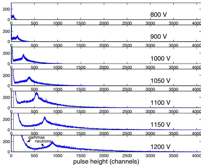
Fig. 6. Energy spectra collected in the 50-straw detector from a moderated  $^{252}\text{Cf}$  source. The detector cathode was biased to the voltage indicated in each panel. The gas mixture was argon-methane (90-10).
