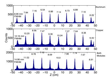
Fig. 7. Position spectra in the direction along the straw axis (z direction), collected in the prototype detector, using a collimator, and at a reactor power level of 50 W. The detector was operated with an argon-methane gas flow, at 1150 V. The full-width-at-half maximum (FWHM) is indicated above each peak. The absence of counts at 0 cm is due to the presence of a fitting that supports the anode wire at the center of each meter-long straw.
