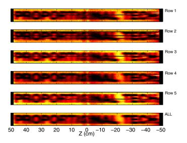
Fig. 9. Two-dimensional image created in the prototype detector, using an acrylic letter target. Separate images are shown for each row in the detector (group of 20 straws), and for all rows combined. Row 1 is the row on the front face of the detector.
