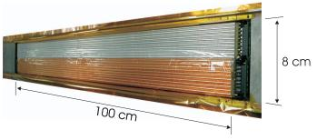
Fig. 3. Aluminum (top) and copper (bottom) prototype detector modules, close-packed to form a  $100 \times 8 \text{ cm}^2$  panel. Neutrons are incident on the face shown. The depth dimension, in the direction of irradiation, is 1.73 cm.
