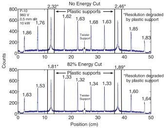
Fig. 10. (*top*) Position spectra collected in a single, 50 cm long straw, 2 mm in diameter, using a slit collimator. (*bottom*) The same spectrum with an upper discriminator level that rejects high energy events (18% of events rejected), resulting in improved resolution. Note the peak broadening in the two peaks positioned over plastic supports, and the clean, narrow inefficient spot in the center, produced by the central wire support.
