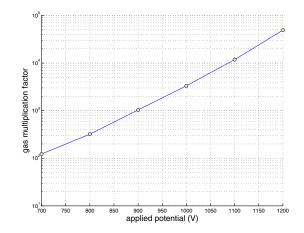
Fig. 5. Gas amplification factor in the prototype detector, filled with 90% argon, 10% methane at 1 atm, as a function of detector bias voltage.
