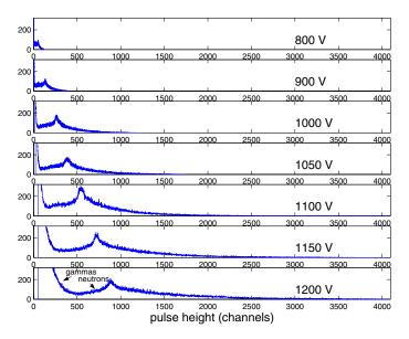
Fig. 6. Energy spectra collected in the 50-straw detector from a moderated  $^{252}$ Cf source. The detector cathode was biased to the voltage indicated in each panel. The gas mixture was argon-methane (90-10).
