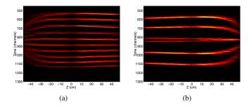
Fig. 8. (a) Correlation between the timing of signals and the corresponding location of neutron interactions along the length of the prototype detector. Each band represents events from one of the ten columns making up the module. (b) Correlation between the timing of signals and the corresponding location of neutron interactions along the length of the prototype detector. Each band represents events from one of the five rows making up the module.
