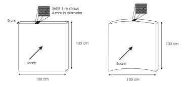
Fig. 1. Neutron area detectors composed of dense-packed  ${}^{10}B_4C$  lined straws, showing a flat panel configuration (left) and a curved panel (right) whose curvature matches the radius of the scattering geometry.
