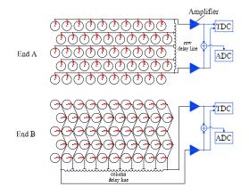
Fig. 4. Electronics setup for straw readout, showing circuitry connected to the two respective ends of each module.
