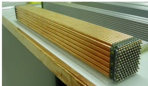
Fig. 6. A small-scale prototype detector was used to evaluate the source detection and localization algorithm. The prototype consisted of 136 B_4C -lined copper straws, each 40 cm long and 4 mm in diameter.
