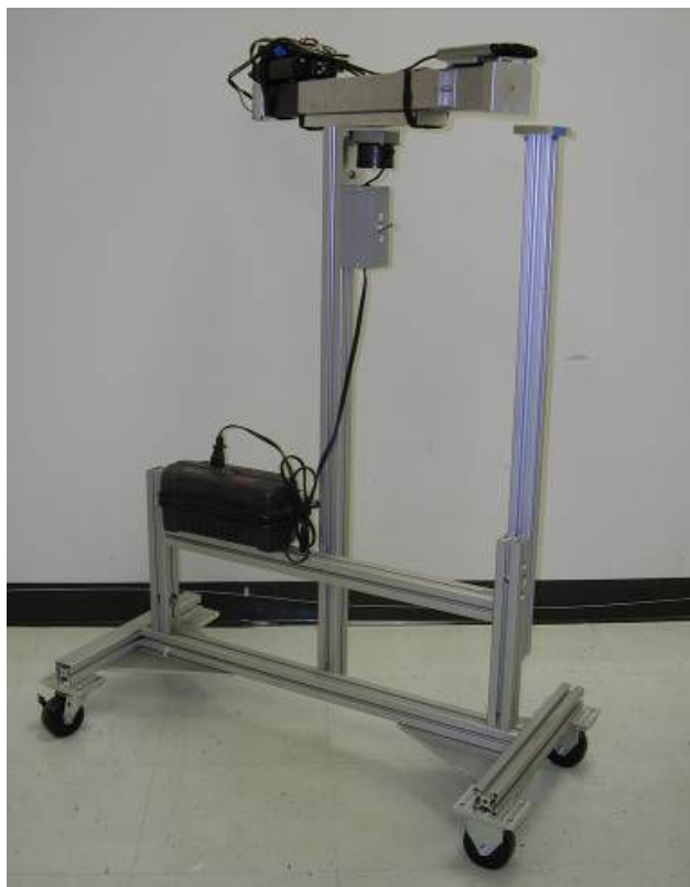
Fig. 8. An aluminum cart was used to support the prototype detector during experiments, and to enable motorized rotation.
