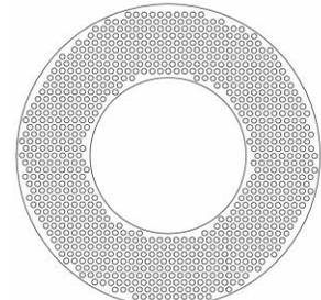
**Figure 3. Cross sectional drawing of moderator showing 804 holes, to accommodate an equal number of BCS detectors.**
