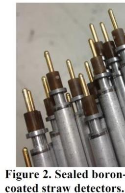
**Figure 2. Sealed boron-coated straw detectors.**
