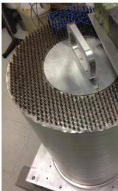
**Figure 1. Prototype straw-based neutron coincidence counter.**
