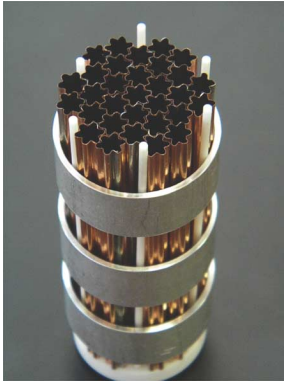
Fig. 8. Prototype 31 Star1 straw detector during assembly.
