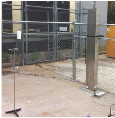
Fig. 2. NDM testing setup, showing the detector supported against the fence, on the right, and the moderated source supported on a stand, on the left.
