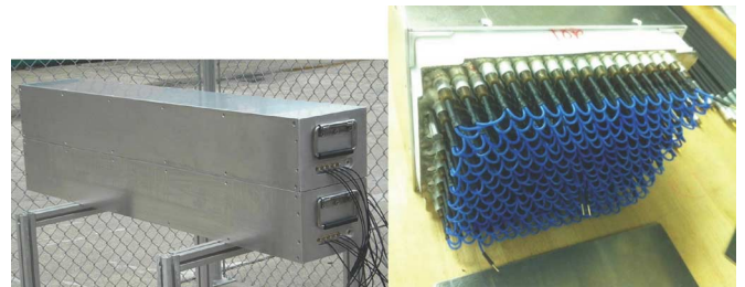
Fig. 4. Prototype neutron detection module.
