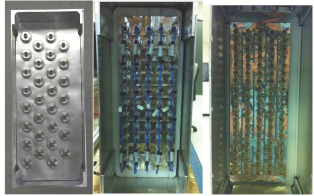
Fig. 1. Portal modules with 30/15 mm straws (left), 60/7.5 mm straws (center), and 95/4.4 mm straws (right).
