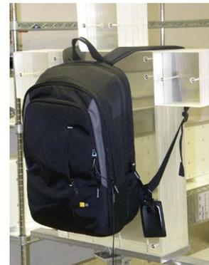
Fig. 5. Backpack radiation detector on torso phantom.
