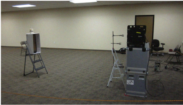
Fig. 4. Experiment setup with a ^{252}\text{Cf} source, shown on the left, supported 2 m away from the detectors.
