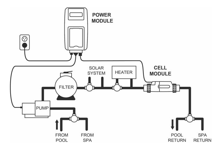
7.1.2 **Figure 1 -** Installation Schematic.
