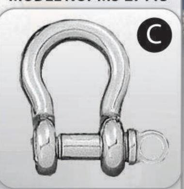
SCREW PIN ANCHOR SHACKLE S.S. T316, PRECISION CAST LOAD RATED, DIMENSIONS MEET FED. SPEC.: RR-C-271D, TYPE IV A, CLASS 2
