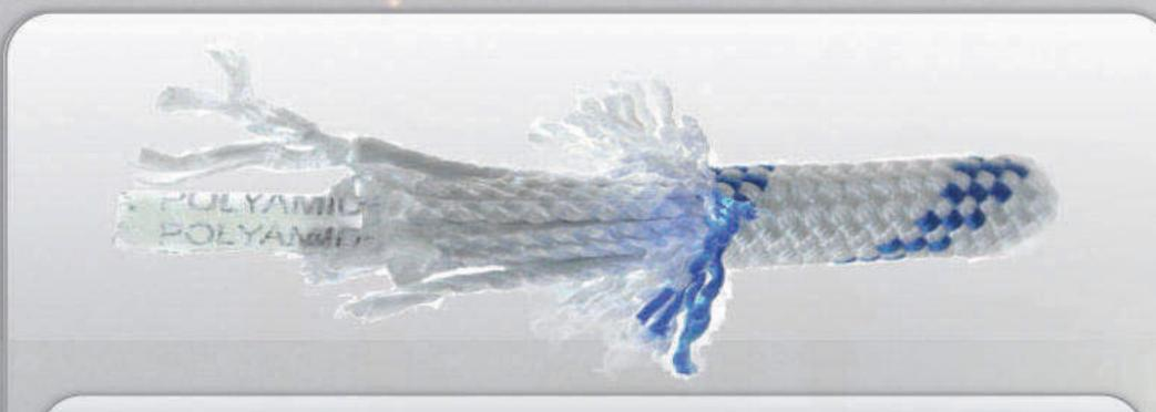
Static kernmantel ropes made from polyamide nylon yarn with UV stabilisation treatment in the full cross section of the yarn. The yarn is thermostabilised at different stages of production and treated for better handling and performance when wet. These ropes have good resistance to repeated falls and are wear resistant.
