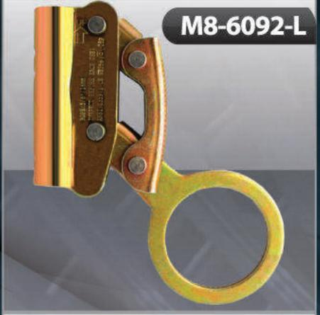
Manual rope grab with a large, mobile eye. Easy to press or release to move along. Built for simple yet reliable operation and positioning. Ideal choice for use with roof kit rope in climbing or slope operations. Designed to be used for 5/8" rope. Meets ANSI Z359.1 standards.
