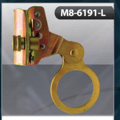
Self-tracking and locking steel rope grab. Designed for use with 5/8" ~ ½" (12 ~ 16 mm) three strand rope. Built for simple yet reliable operation and positioning. Meets ANSI Z359.1 standards.
