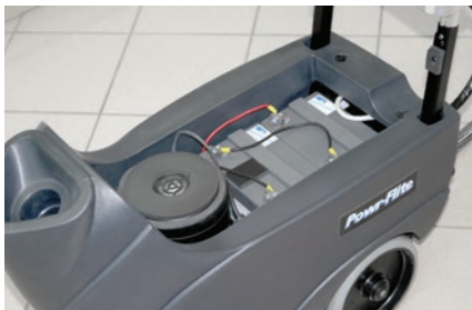
Easy access to motor and battery
