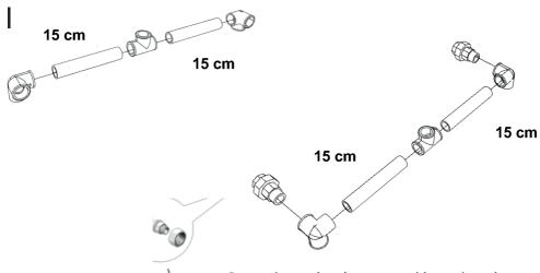
Once the union is screwed into the piece, then loosen the nut so that the end of the union becomes free.
