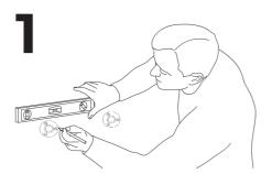
Mark the holes in the "Flanges" on which surface the shelf should be placed.
