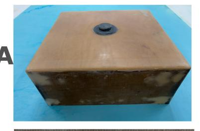
Drain Knockout attached to bowl mold.
