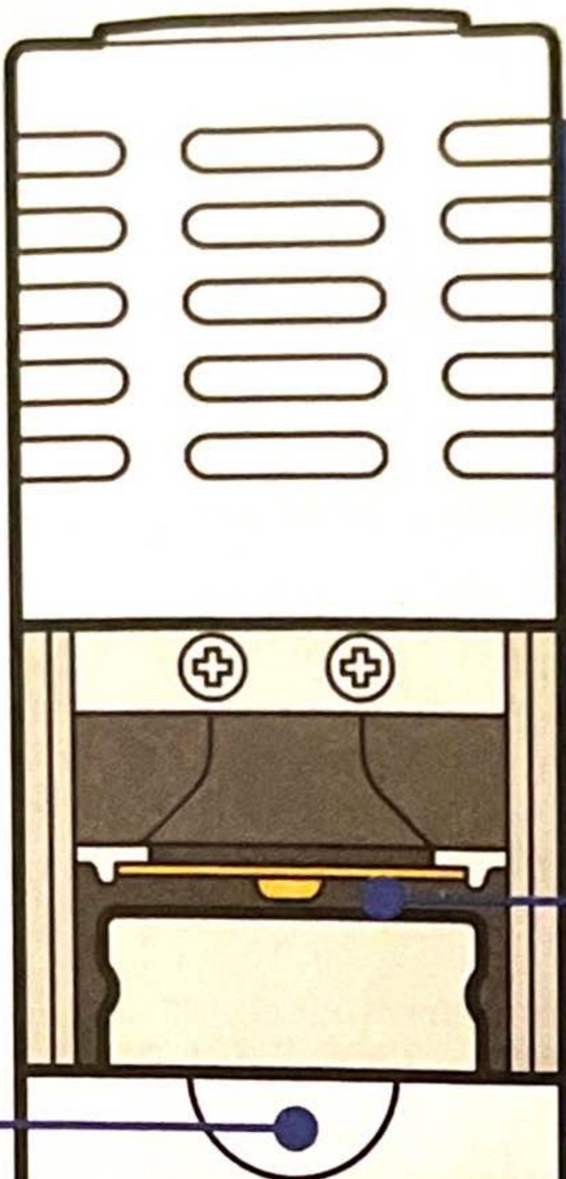
Slide down rear cover for easy access to the battery
