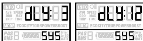
Delay time of battery power interface
