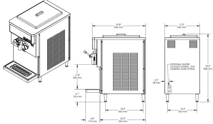
Minimum Wall Clearance Both Sides and Back -6 inches (152 mm)
