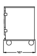
**GENERAL:** Cabinet shall be constructed with a aluminum exterior and interior. All double wall construction insulated with high density fiberglass insulation. All exterior surfaces shall be ground and polished to a #3 finish.
