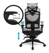
The height adjustment lever is on the right armrest. Body weight would lower the seat when the lever is pressed. Seat will rise when no weight is applied to the chair upon the pressing of the lever.
