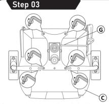
Remove the bolts and install the tilt-mechenism. 用部件上的螺絲把托盤裝上.
