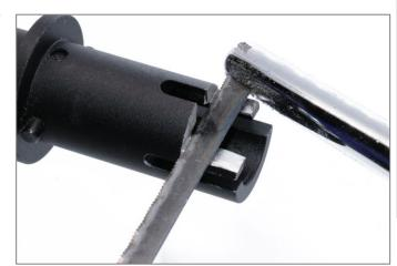
Take a sanding tool to remove 21B any bit or burs. Use sandpaper to clean up the edges and smoothen sharp edges. Wipe out with wet paper to clean out bits of metal and shavings.
