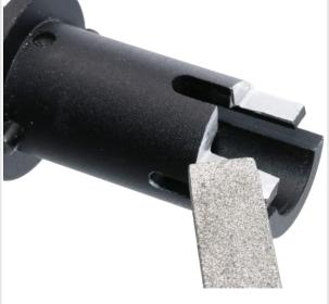
22B Once completed, try testing the TDC kit & Chamber into the outer barrel. Repeat 20 and 21 incrementally until it fits in nicely like the demo below. When complete install the outer barrel back into the handguard followed by the hop-up unit.
