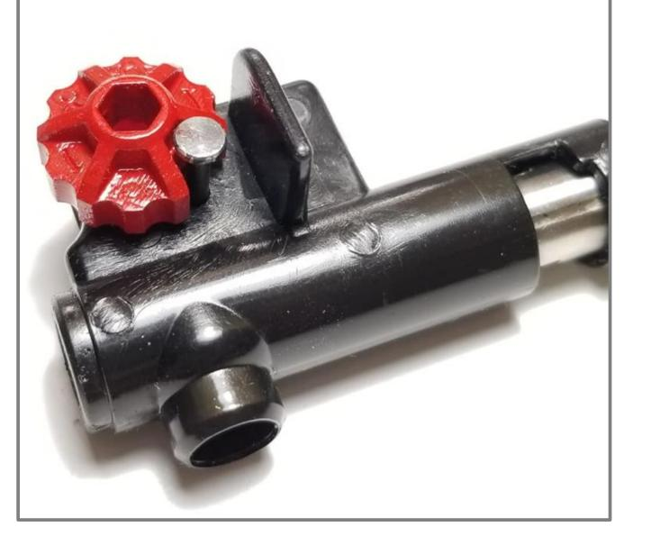
Hold/press the hop-up arm to align the holes together enough to insert the pin into place.
