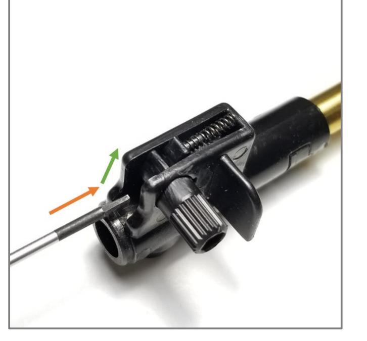
Next to remove the hop-up Arm. Use the screw driver to insert into the hop-up unit, underneath the adjustment knob. Tilt your screwdriver and push up. The hop-up arm will pop out.
