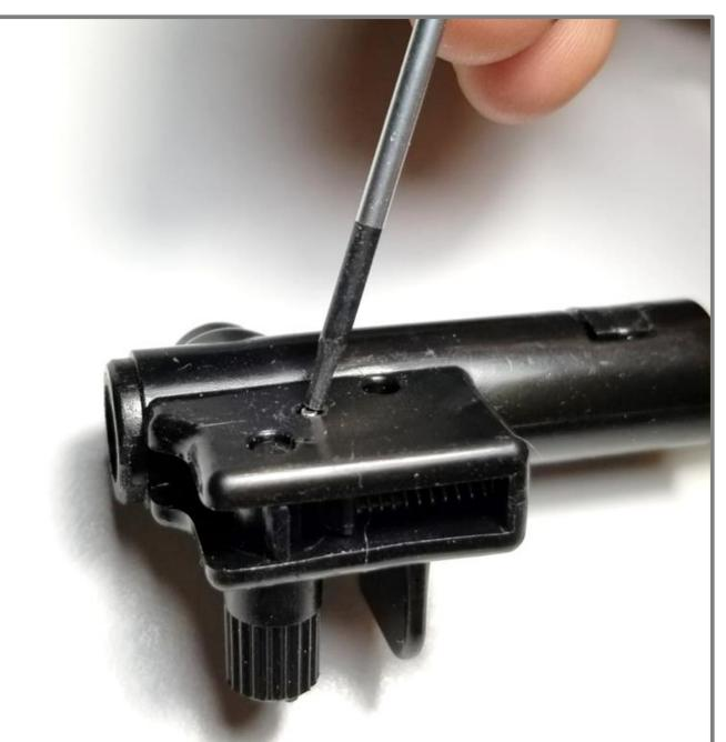
Remove the hop up arms pin. Use you can use a thin screw drive to punch it through
