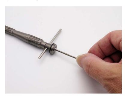
5. The bearing and screw should now be removed. It is possible that the screw could still be jammed inside the bearing due to a tight fit. This is not a problem, as we include an extra screw in the upgrade kit in case you cannot remove the original screw from the bearing.
