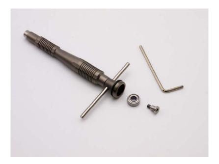
6. Insert the new screw into the ceramic bearing, then install them into the bearing housing and tighten the screw. Do not overtighten the screw, or you may strip the socket.
