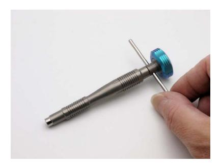
2. Unscrew the end cap and remove it from the bearing mount.
