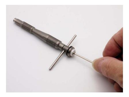
7. Thread the end cap back onto the bearing housing and tighten. Remove the torq bar and you are ready to spin!
