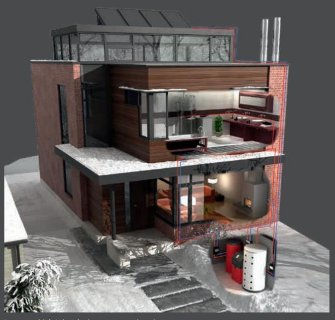
A cutaway model of a hydronic fireplace insert integrated into a heating system.
