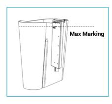
• Fill the tank to the 'max' mark with either tap water or distilled water.
