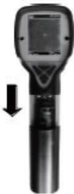
2. Take out the battery holder to replace with new batteries (Pay attention to the anode and cathode during installing).
