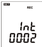
1. Fig.1 Set interval time for data logging.
