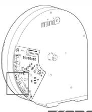
Connect the sensor in the electronic board with the provided cable.
