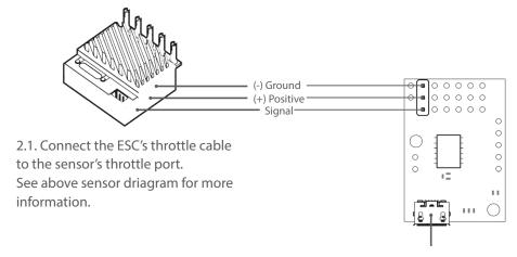
2.2. Connect the sensor to the PC with a mini-b USB cable.
