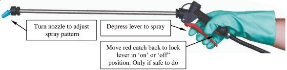
After spraying is completed, drain unused chemicals from the tank. Rinse the tank with clean water then operate the sprayer with clean water in the tank to clean out the pump, hose and spray lance. Do not leave chemicals in the tank as they may crystallize or form solids in the pump, spray lines and block the filter.
