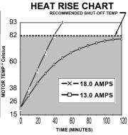
The heat rise chart indicates (in the greyed area) the conditions where this pump can operate under a continuous duty cycle when ambient temperatures are 21° Celsius or less. **Note** when current draw is greater than 13amp at 21° the duty cycle is rated as intermediate
