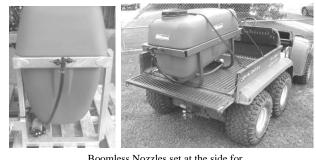
Boomless Nozzles set at the side for Tray Mounting
