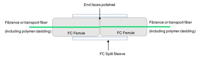
Fibrance fiber terminated in an FC connector is ready for attachment to a single-color or multi-color laser as pictured to the right.
