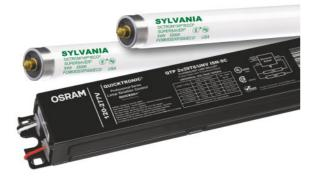
QUICKTRONIC SYSTEM 59 ISN UNV electronic T8 ballasts offer several advantages:- Operate OCTRON T8 lamps with maximum efficacy and high lumen output- Over 30% energy savings when compared to F96T12 magnetically ballasted systems- Longer Lamp Life: provides 50% longer lamp life compared to standard magetic T12 slimline systems- Parallel Circuitry: keeps remaining lamp lit if one goes out- Small Can Enclosure for: - low profile fixture design - transportation, inventory and ergonomic benefits
