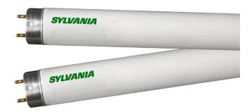
OCTRON VIVID VALUE ECOLOGIC T8 lamps provide exceptional color rendering with a 90 CRI for color critical applications and outstanding value for the price oriented end-user. Available in a wide range of color temperatures, these lamps have a rated lamp life of up to 22,500 hours on instant start and up to 27,000 hours on programmed start ballasts at 12 hours per start. Pair OCTRON VIVID T8 lamps with QUICKTRONIC electronic ballasts for coverage by the comprehensive QUICK 60+
