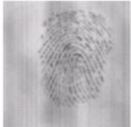
This is an example of a user not applying enough pressure. Although the core is centred, you can see that the image coverage is very poor.
