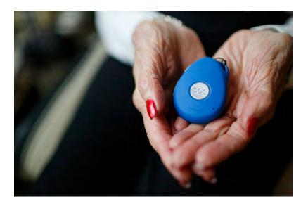
Mobile help alert devices essentially act like a simplified cell phone and are assigned their own phone number. There is no need for a landline, base console, or existing phone line, so all the technology is completely self-contained within a pendant that can be worn by the user. And unlike landline-based devices, cellular help alerts can be pre-programmed, so there is no installation required by the wearer. Just take the pendant out of its box and turn it on.
